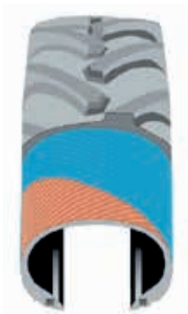
Bias tire construction: the cords are placed diagonally with certain degrees for the rotation direction of a tire.
