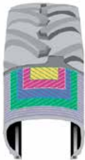
Radial tire construction: The cords are replaced towards the tire center with 90 degrees.
