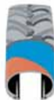
Bias tire construction: The cords are placed diagonally with certain degrees to the rotation direction to the tire.
